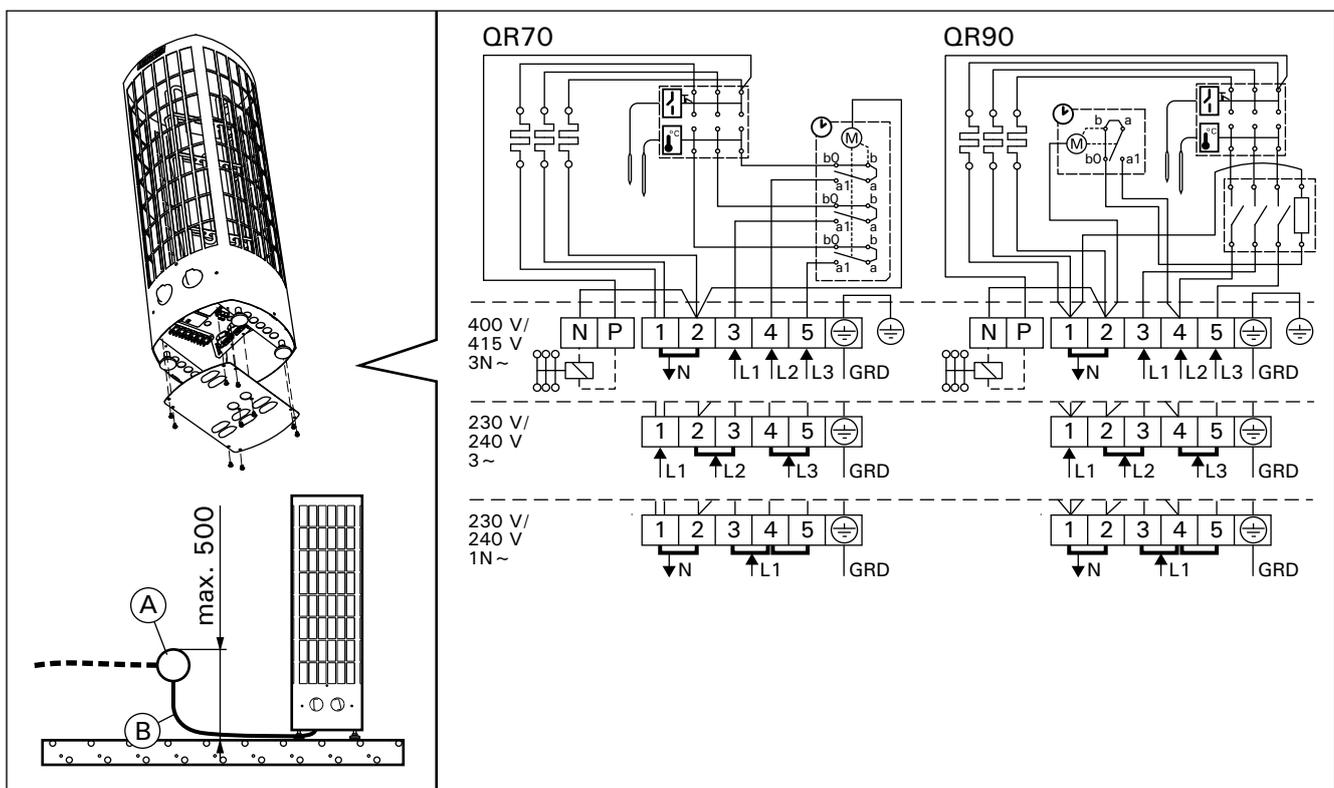
Figure 7. Electrical connections
