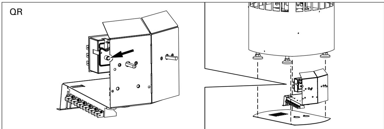
Figure 9. Reset button for overheat protector
