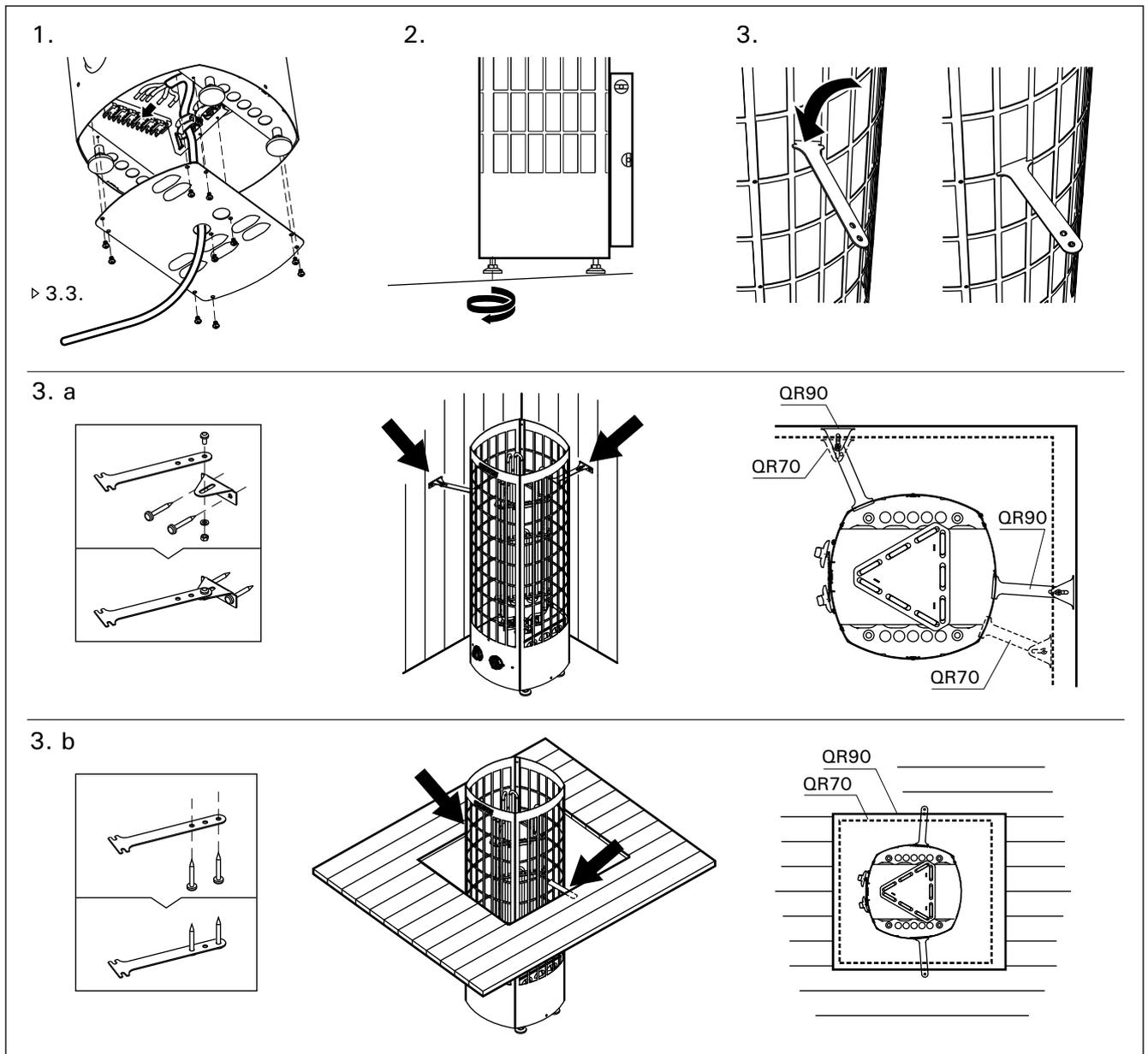
Figure 8. Installing the heater
