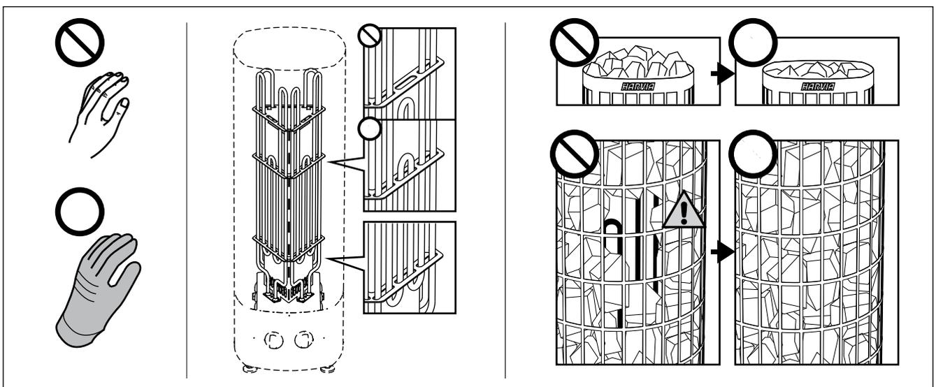
Figure 1. Piling of the sauna stones
