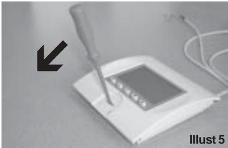
2. Unlock the housing by lightly turning or tilting the screwdriver in the direction of the arrow (Illust 5) and swivel the upper part of the housing upwards.
