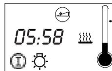
If the device is in humid mode (level „P3=1“) the sauna furnace, vaporiser and sauna lights are operating.
