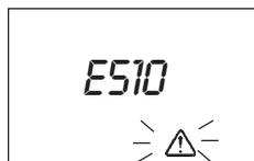
If no water is filled within the set time, the appliance switches the entire sauna off for safety reasons. The error message opposite appears in the display.
