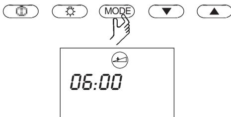
Now you can preset the heating time as required using the ▼ and ▲ setting buttons.
