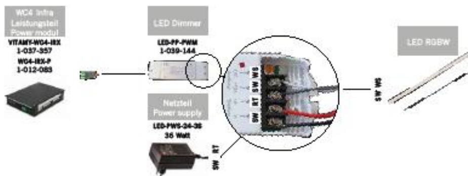
Fig. 42: Connecting the LED strip to the control unit
